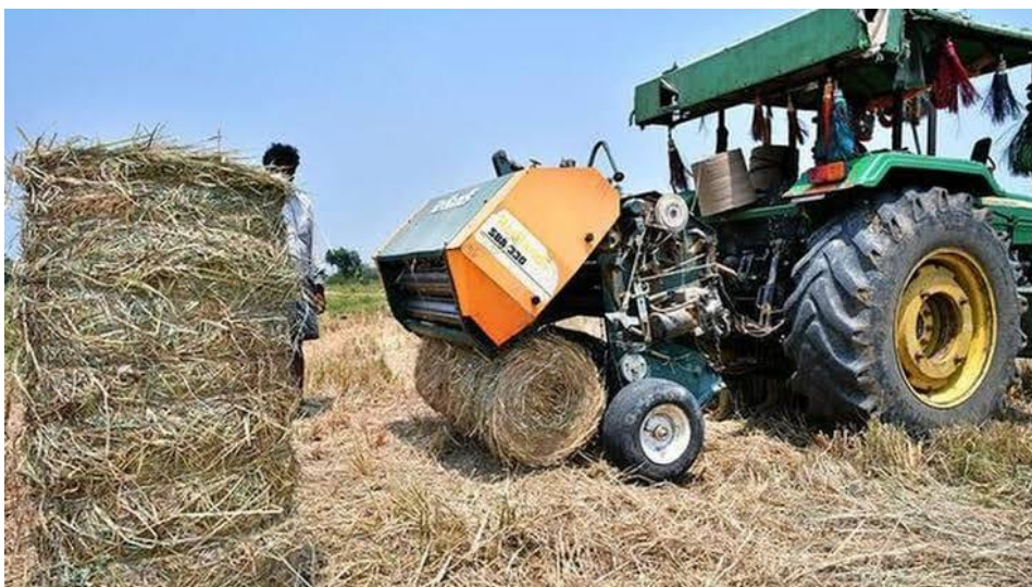
Paddy straw was converted to balers by using Rice baler machine in KLEF fields, Gundimeda, Andhra Pradesh
