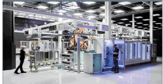
Figure 8-8. DC micro grid demo cell AREUS (Automation and Robotics for European Sustainable Manufacturing)
