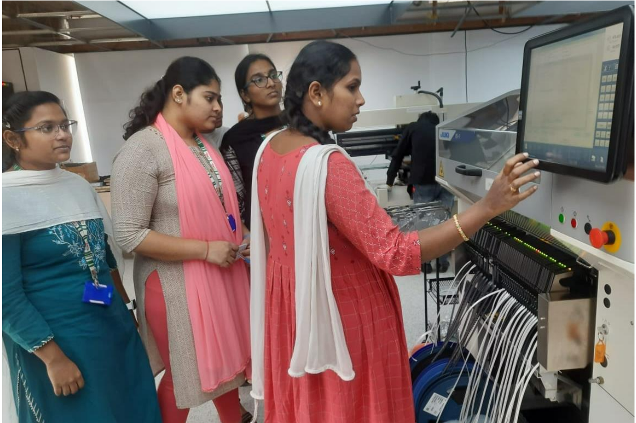
PCB Components Automatic Pick and Place Machine
