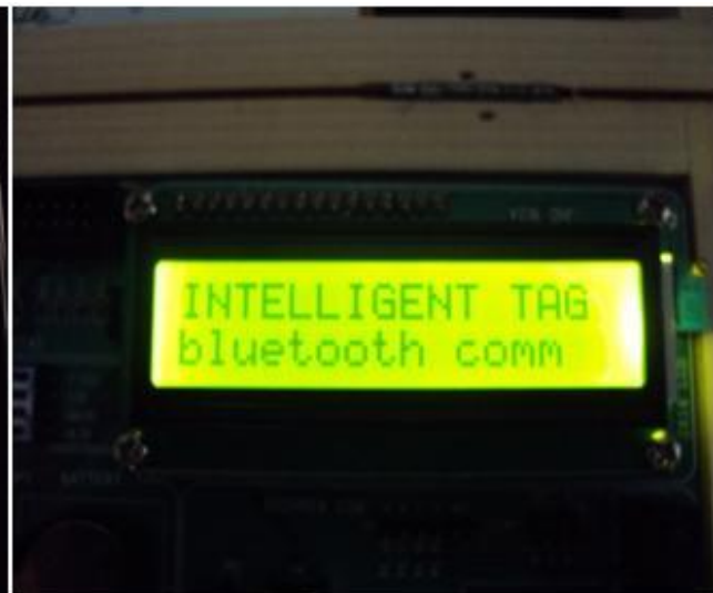
Communication Establishment Data Sent From Mobile Displayed On LCD
