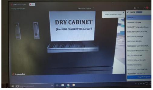
Dry cabinets can eliminate potential defects which caused by humidity in IC packages and printed circuit boards (PCBs). With the introduction of lead-free products, proper handling and preservation of these moisture sensitive components (MSDs) has become more important than ever.
