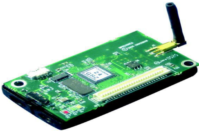
Figure-1- 2.4 GHz IEEE 802.15.4, Tiny Wireless Measurement System
