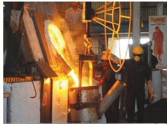
Additionally, students gained an understanding of the core-making machine, witnessing the injection of core sand. In the core preparation section, they examined how to correct a damaged core, which is necessary for placement in the prepared mold. The process of preparing molten metal in an electric induction
