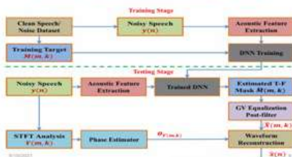
DNN Based Single-Channel Speech Enhancement Technique Using Phase Estimate Based T-F Masking
