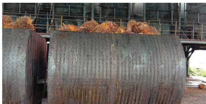
These loaded containers are subjected to sterilization (moist heat) at 5kg pressure. This is done to decontaminate the palm fruits and loosen them as steam passes into them, so that it could be easy to separate the seed from the fruit. Here they use the mesocarp of the fruit is used for the production of oil not the seed.
